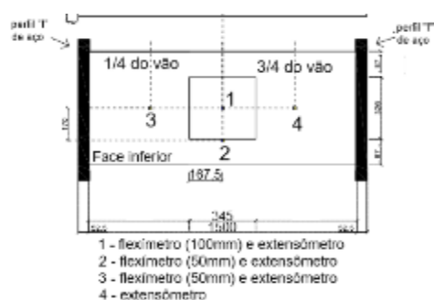
Fig. 8 — Instrumentation of the panels. Source: [1].
